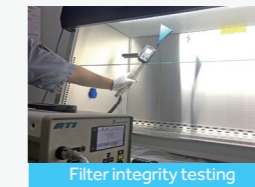
Filter integrity testing
