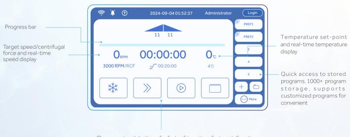
Clear one-touch buttons for fast refrigeration, fast centrifugation, intelligent start-stop and lid-opening button
