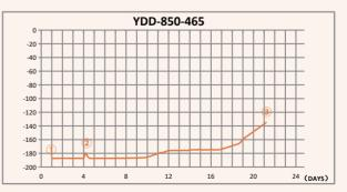
1 Precooling stage when freezer filled to high level 2 Lid open test, -179.4°C max <sup>3</sup> With no liquid nitrogen supply, the temperature maintained below -135°C for 21 days
