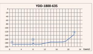
1 Precooling stage when freezer filled to high level 2 Lid open test, -179.2°C max ③With no liquid nitrogen supply, the temperature maintained below -135°C for 22 days
