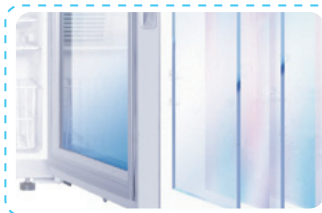
Three-layer tempered glass door, filled with inert gas in the middle, low-E film to effectively reduce the risk of condensation
