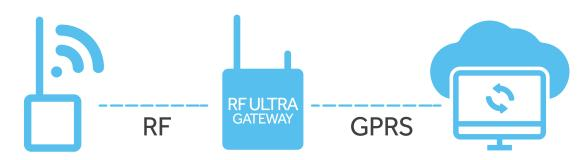
wireless RF transmitters manufactured with bespoke functionality and often sensors around the application chosen infrastructure - Internet, cellular RF Gateway – This device collects data from the transmitters, stores into memory and transfers up to the Realtime Online web server at regular intervals realtime online, web-based software that provides information to the application, plus automated and on-demand reports, alarm notifications, dashboard/information screen etc.
